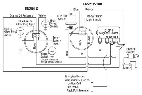
**Note:** Use of the **black wire** on the **EN204-S** and the **518PH Magnetic Switch** (as shown in the diagram) is required for engine shutdown.
